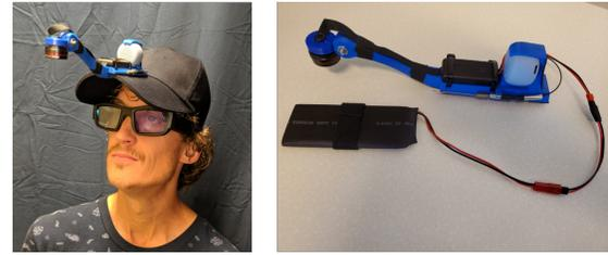
(a) Final hands-free device prototype (b) Close-up view of 3d-printed hat mount for fisheye camera and speaker/mic
